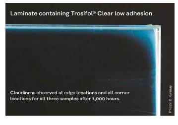
If we were to apply this test to glass on its own, we would not see any adverse effects; with glass being a relatively inert material. However, this may not be the case for the panels fabricated using interlayers, especially if they are deployed in open-edged laminated panels.
