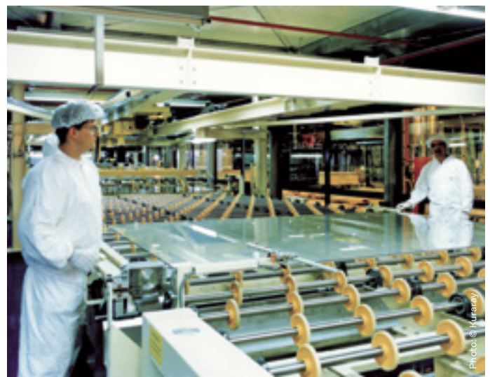
➤ Positioning of PVB film
