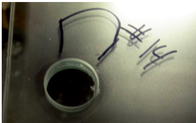
FIG 32 • Prepress too cold
