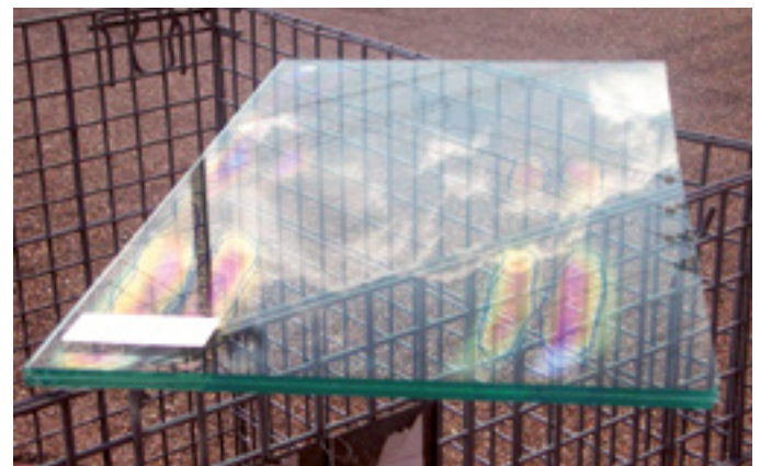
FIG 23 • Laminate showing optical distortion
