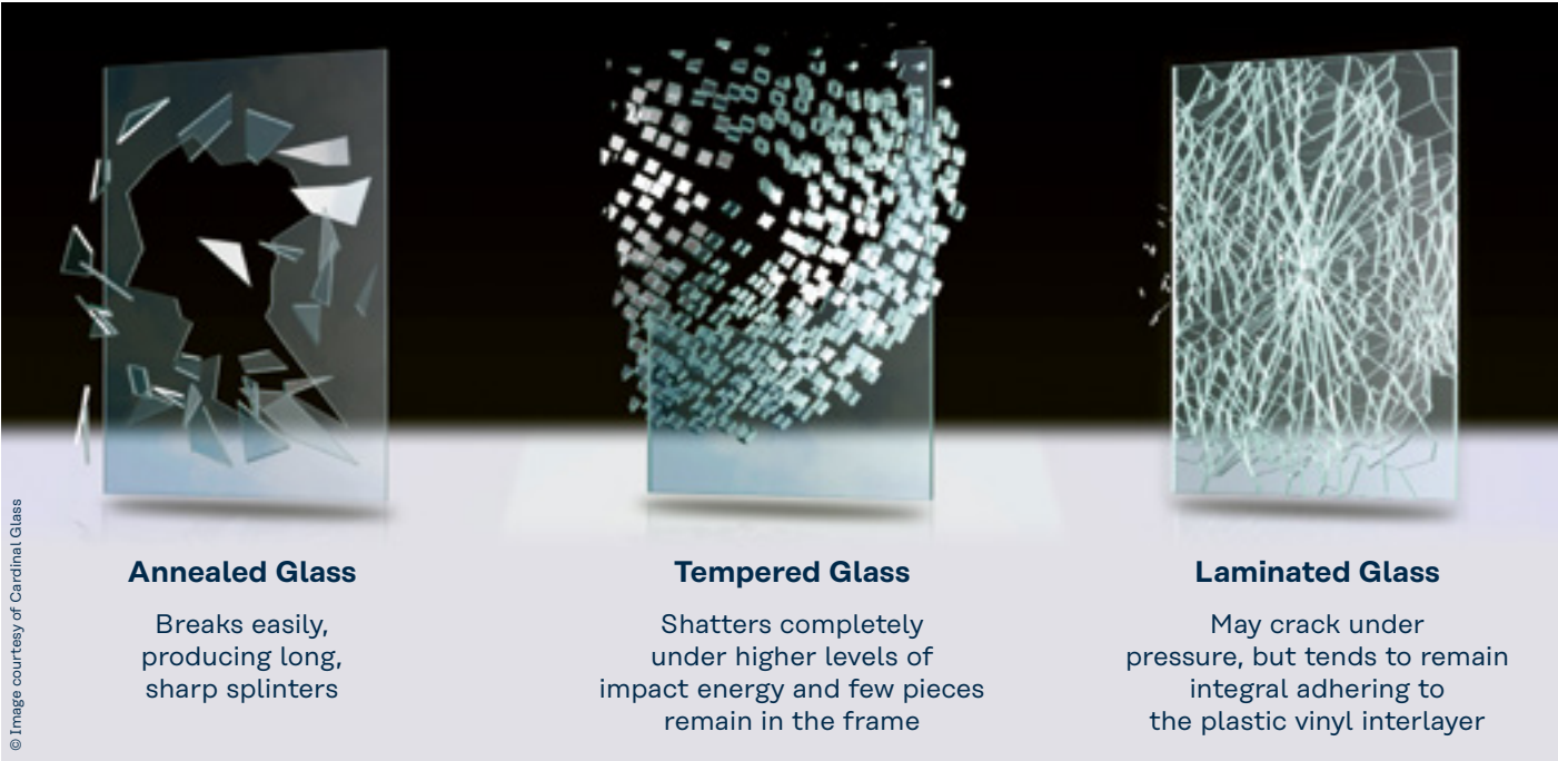
Comparison fracturing of annealed, tempered (or heat-strengthened) glass vs. laminated glass made of annealed glass
