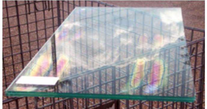
FIG 23 • Laminate showing optical distortion
