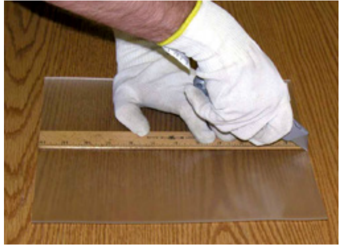
FIG 9 • Cutting SentryGlas Xtra®: Score pattern using a utility knife
