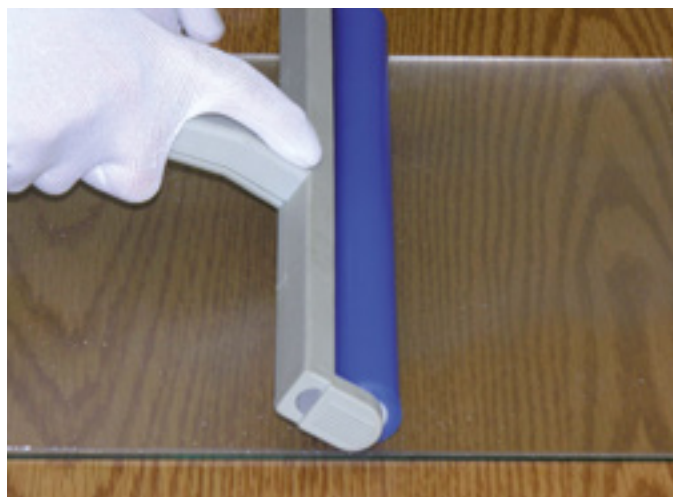
FIG 11 • Cleaning SentryGlas® with contact roller
