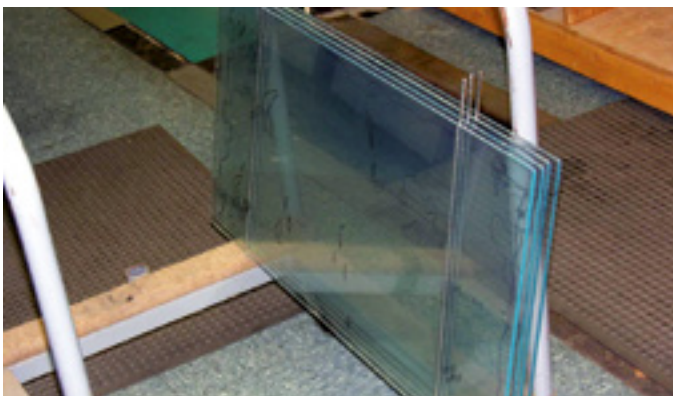
FIG 22 • Improperly racked laminates
