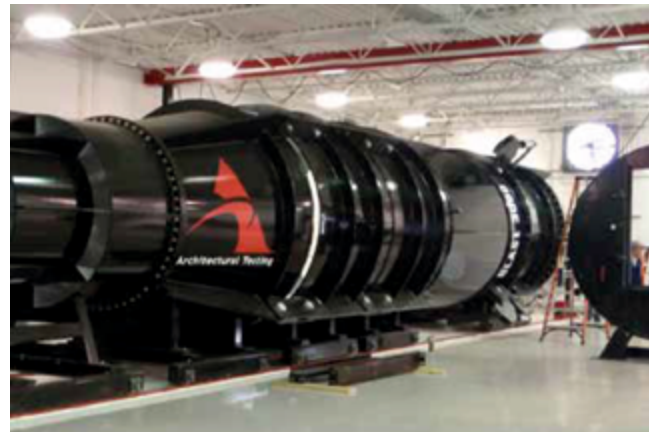
➤ A shock tube focuses a blast-level pressure wave against a mounted glass sample.
