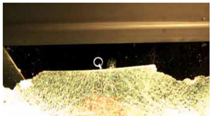
Fig. 4: EVA laminate provided no "Fall Through" resistance
