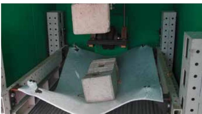
Fig. 12: 0.89 Ionomer laminate collapsed at 200 Kg
