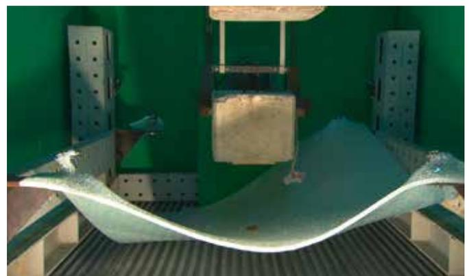
Fig. 11: Broken Stiff PVB laminate collapsed at  $50\text{ }^{\circ}\text{C}$
