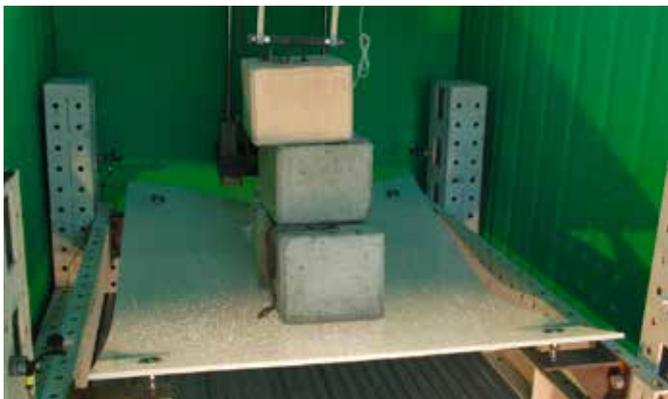
Fig. 8: 400 Kg load on Ionomer laminate at  $21\text{ }^{\circ}\text{C}$
