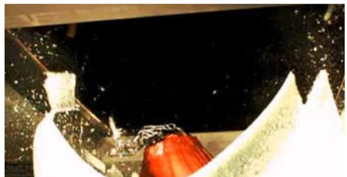
Fig. 6: Stiff PVB laminate provided no "Fall Through" resistance
