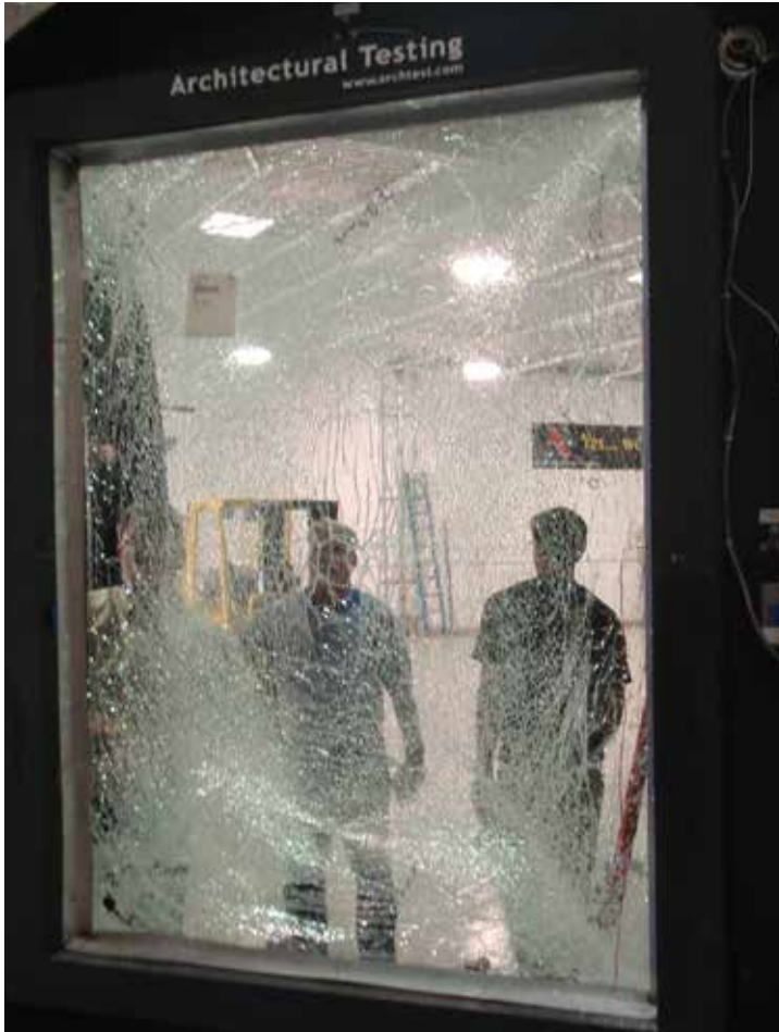
A laminated glass panel is inspected after shock tube blast testing (above), to assess glass fragmentation.
