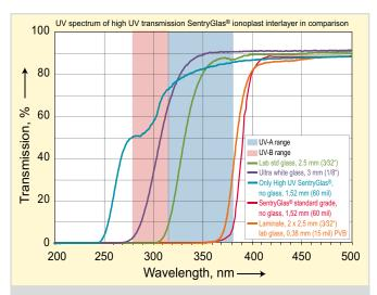
The Tropenhaus renovation uses insulated, doubleglazed panels with the inner glass laminated for safety performance. The inner laminates are made with a special grade of SentryGlas® for high UV transmission, supporting plant health by letting through more natural light.
