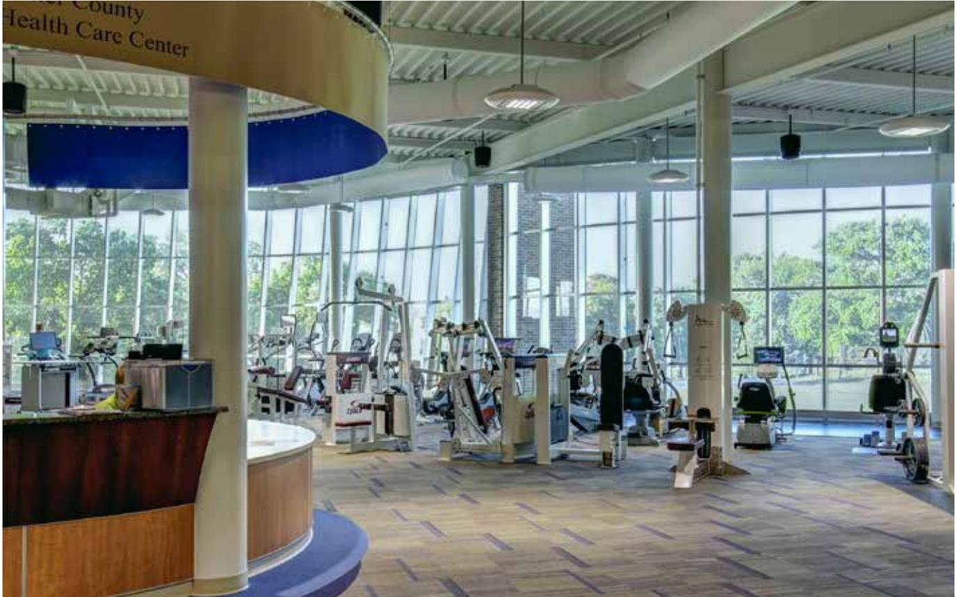
*The curtain wall, which employs SageGlass® electrochromic glass and SentryGlas® ionoplast interlayers, controls solar gain and glare without impacting on the internal brightness of the open spaces.*
