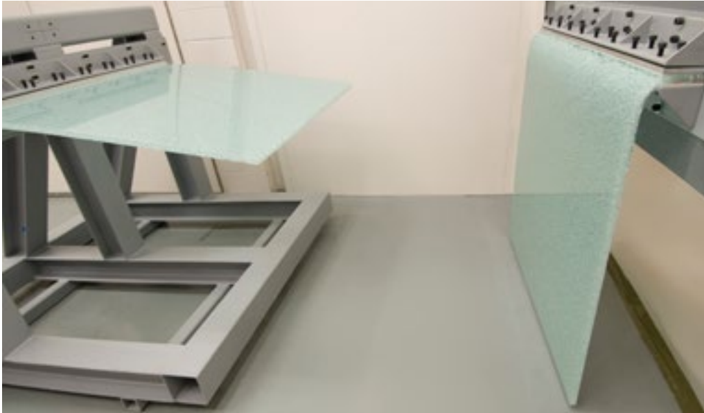
SentryGlas® vs PVB - post-glass breakage
