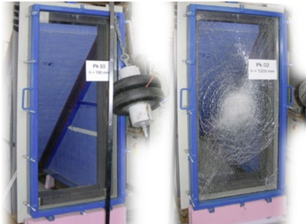
Impact test EN 12600 by University of Applied Science, Munich, Germany, 2009.
