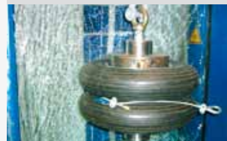
Pendulum test in accordance with EN 12600
