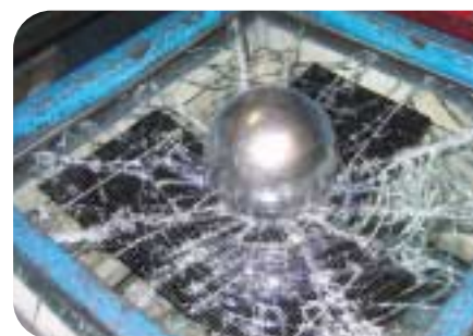
Ball drop test in accordance with DIN 52338
