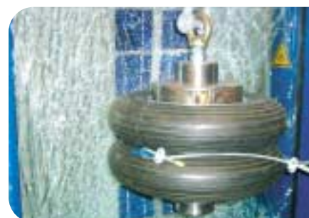
Pendulum test in accordance with EN 12600
