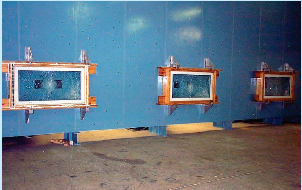
Test specimens mounted on the wall for impact and cyclic testing. Source: NCTL Laboratories of an air cannon.
