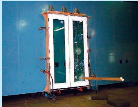
Impact Testing Source: NCTL Laboratories
