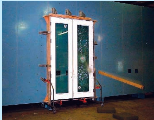
Impact Testing Source: NCTL Laboratories
